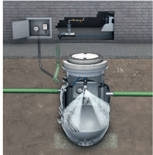
Installation example shows ACO LipuMax P-DA NS 4 with a top section unit for load class B 125
