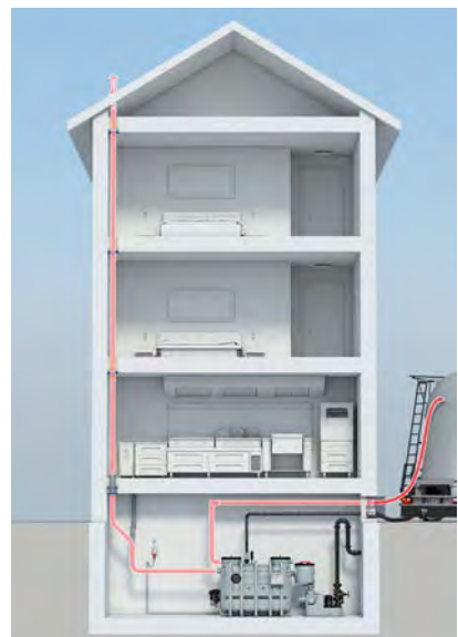
Pendulum gas line connected to grease separator
